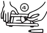
Apply glue to the board and patch using a brush or other applicator. Make sure the glue is evenly and completely distributed on the board and patch. Allow the glue to dry for 5 minutes.
